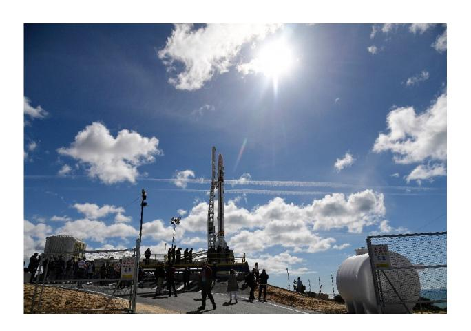
PLD Space's MIURA1 sub-orbital launcher is intended to carry out up to four missions a year.
