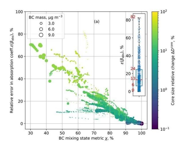
Error in absorption coefficients after composition averaging for dry particles. Each marker represents an aerosol population. Color shows the change in black carbon (BC) diameter due to composition averaging; marker size shows
