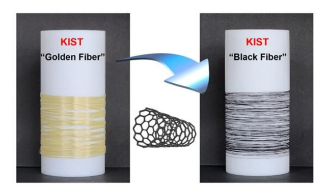
"Black fiber" created from a mixture of aramid polymers and carbon nanotubes. Credit: Korea Institute of Science and Technology
