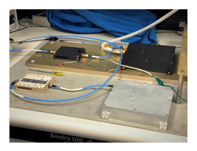
In a Goddard Space Flight Center laboratory, navigation experts test the LuGRE payload's GNSS receiver and low noise amplifier. Credits: NASA / Dave Ryan
