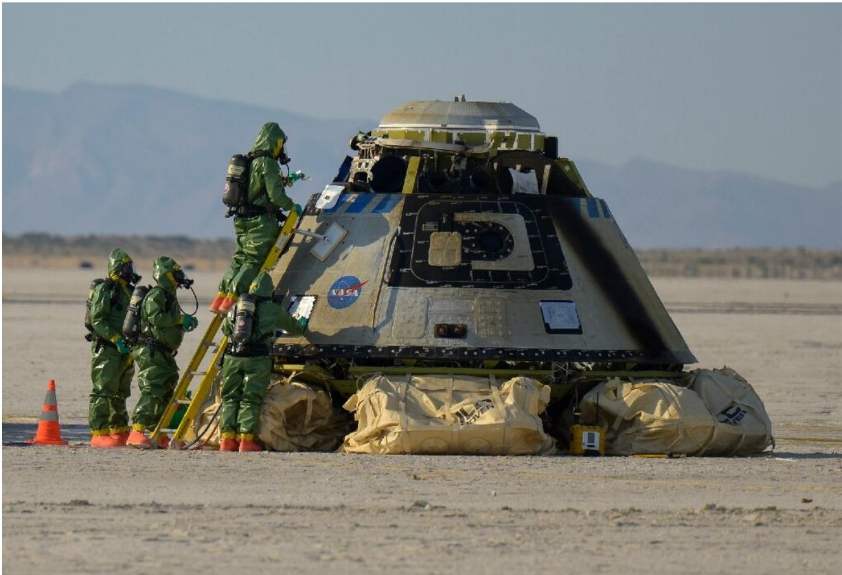
Boeing's CST-100 Starliner space capsule after landing at the White Sands Missile Range following an unmanned May 2022 test flight.
