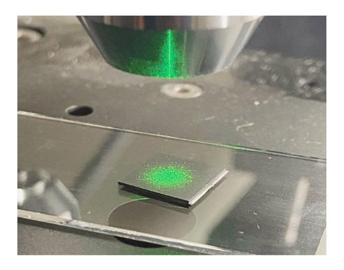
With laser light and the so-called Raman effect, small material samples can be analysed and show whether, for example, traces of pollutants are contained. The substrate on which the sample lies plays a decisive role here. Credit: Cenk Aktas / Josiah Shondo
