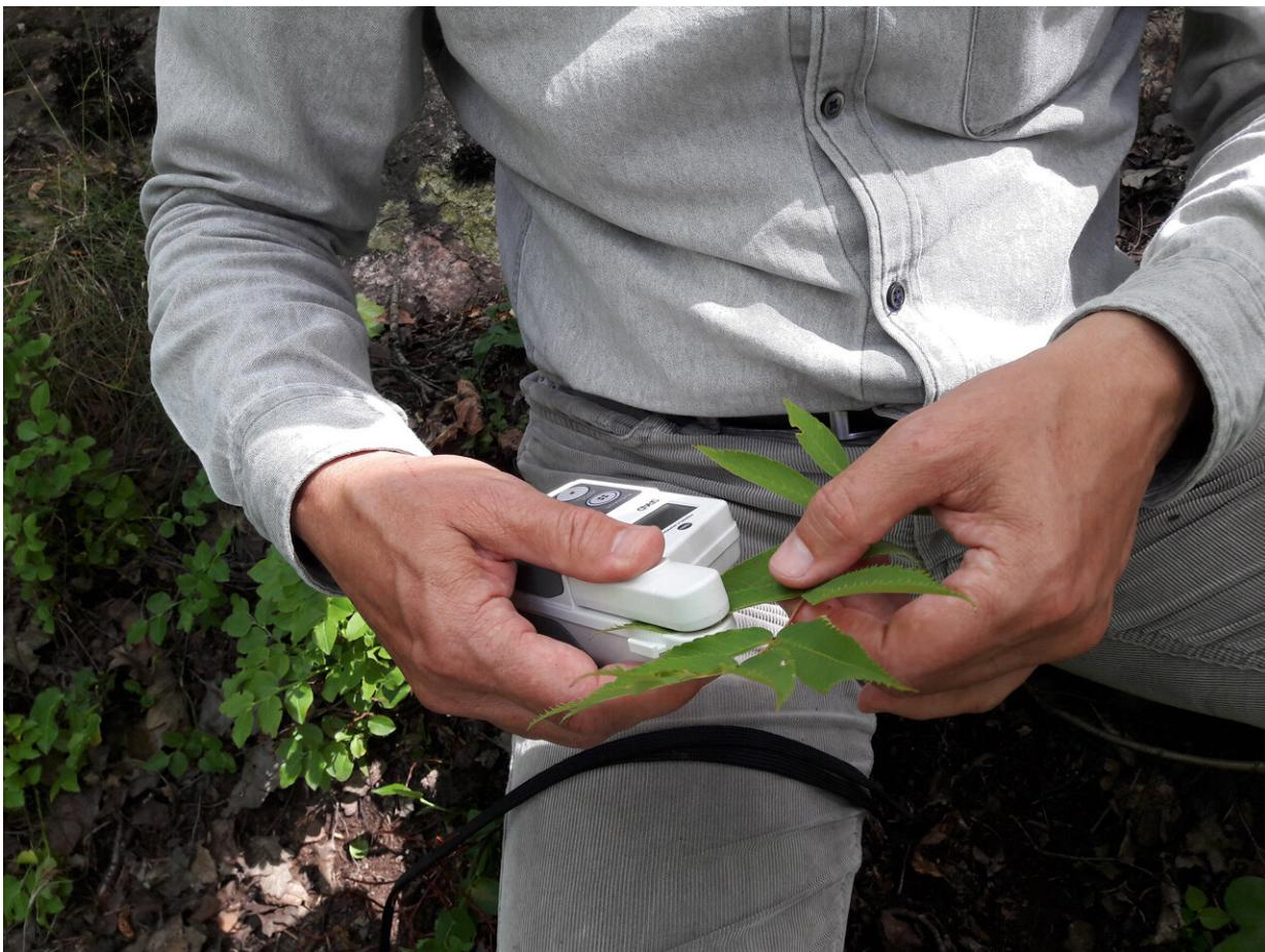
Measurement of chlorophyll in leaves using a chlorophyll measurement device called a SPAD. The measurement is done using light, leaving the leaf undamaged. Credit: Jenny Klingberg
