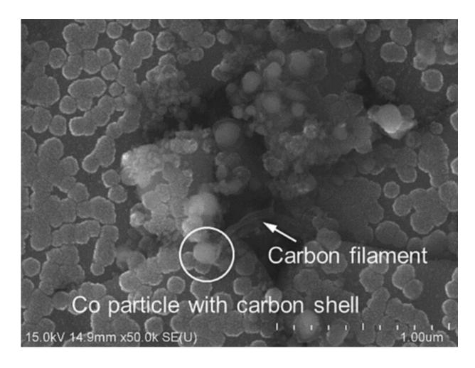
Carbon filaments grown from cemented tungsten carbide. Credit: Toyohashi University of Technology
