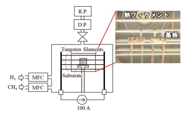
Conceptual diagram of HF-CVD deposition apparatus. Credit: Toyohashi University of Technology
