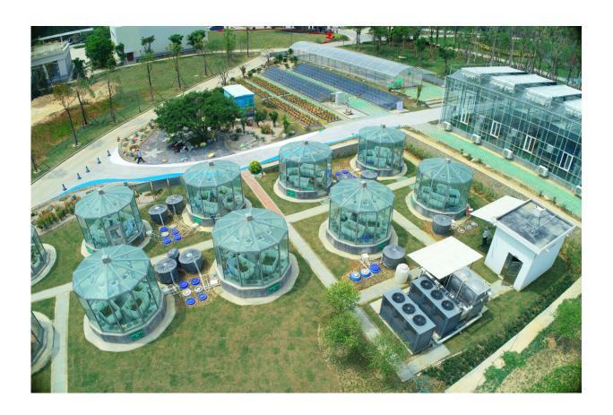
The system controls the atmospheric carbon dioxide concentrations, flooding time, temperature, light, humidity and other environmental factors suitable for the study of costal wetland ecosystems global change manipulations. Credit: Jialin Zhang from Xiamen University
