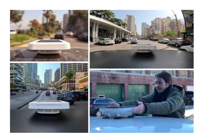
MIT researchers have made an open-source version of the "City Scanner" mobile pollution detector that lets people check air quality anywhere, cheaply. Pictured are some examples of the latest version of the device, called Flatburn, as well as a researcher attaching a prototype to a car. Credit: Massachusetts Institute of Technology
