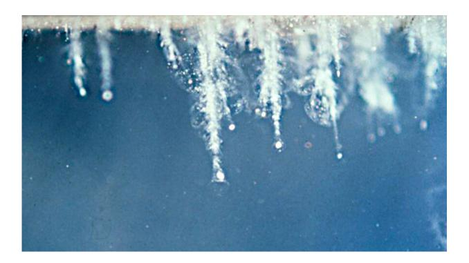
While not part of this study, this photo taken with a microscope shows the impact paths and bodies of small particles of comet debris from U.S. space agency NASA's Stardust mission in 2004. The aerogel helps decelerate the particles without destroying them in the process. Credit: ©2023 NASA/JPL CC-0
