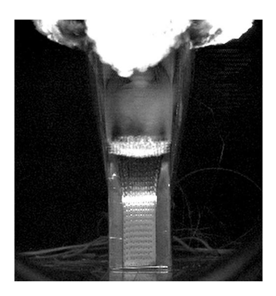
High-speed camera frame of a detonation wave propagating through a liquidfilled, 3D-printed, high-explosive lattice. The lattice was "switched on" when it was filled with water. Credit: Los Alamos National Laboratory
