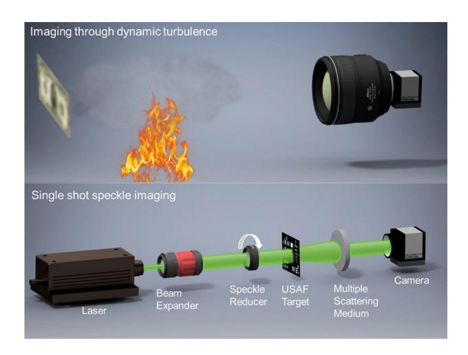
Experimental setup. Two separate setups were used to demonstrate our method in (1) imaging through dynamic turbulence generated by fire and (2) single shot speckle imaging through multiple scattering. Credit: UNIST
