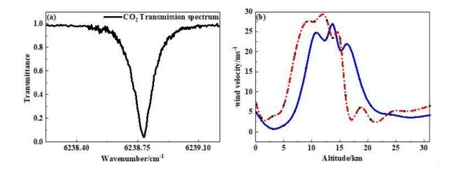
(a) The measured atmospheric transmission spectrum; (b) The prior wind profile (blue curve) and the inverted wind profile (red dotted line). Credit: Li Jun
