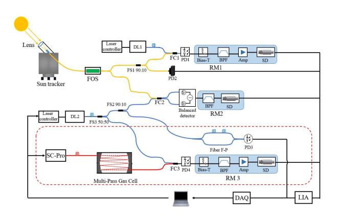
Schematic diagram of near-infrared laser heterodyne radiometer. Credit: Li Jun
