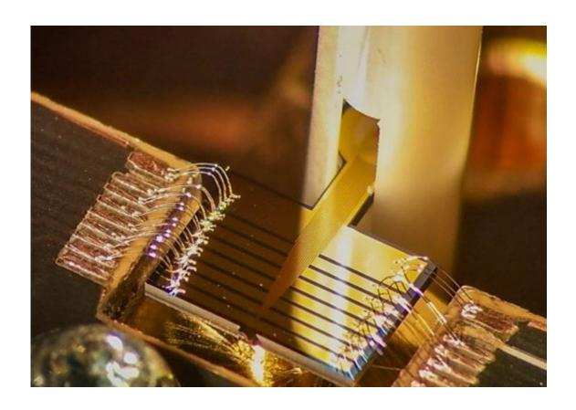
Using these sensors, scientists were able to generate a secret key at a rate of 64 megabits per second over 10 km of fibre optic cable. Credit: M. Perrenoud - G. Resta / UNIGE
