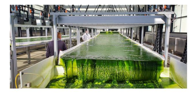
Pilot plant photobioreactor for oleaginous algae biomass production at the TUM AlgaeTech Center. Extracted lipids from biomass are used for third generation aviation biofuels. Credit: Thomas Brück/TUM (CC-BY 4.0,
