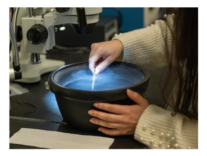
Maria Solares, first author on both papers, demonstrates the transfer of a specimen in liquid nitrogen in preparation for imaging in the cryo-electron microscopy instrument. Credit: Jeff Xu/Penn State.
