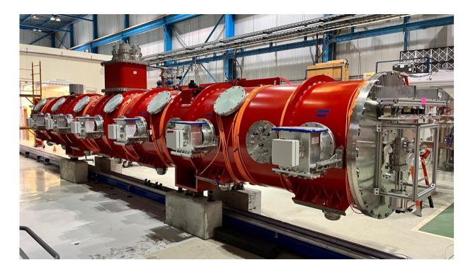
The fully assembled prototype high-beta 650-megahertz cryomodule. Four of these will make up the final stage in Fermilab's new linear accelerator. Credit: Saravan Chandrasekaran, Fermilab
