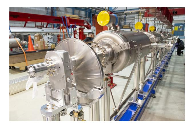
The cavity string for the HB650 cryomodule after being assembled in April 2022. These cavities comprise the heart of the new cryomodule. Credit: Lynn Johnson, Fermilab
