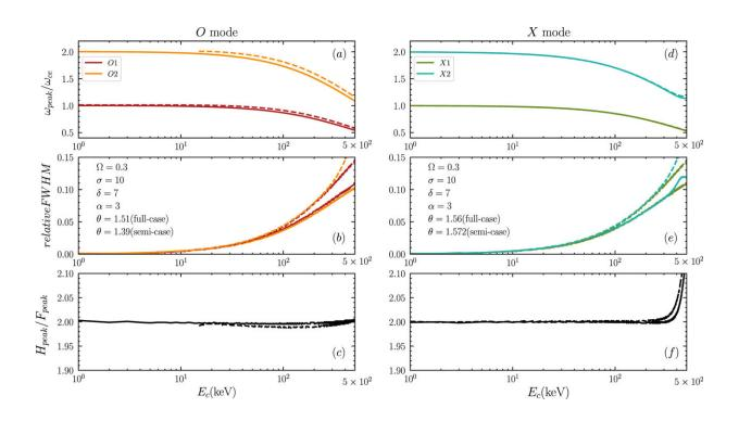
Peak frequency  $\omega_{peak}$ , relative frequency FWHM  $\omega_{width}/\omega_{peak}$ , peak frequency ratio between the harmonic and fundamental frequency  $H_{peak}/F_{peak}$  vs. cutoff energy  $E_c$ : O1 (2), fundamental (harmonic) waves in the O mode; X1 (2), fundamental (harmonic) waves in the X mode; solid and dashed lines denote the "full case" and "semicase," respectively. Credit: *The Astrophysical Journal* (2023). DOI: 10.3847/1538-4357/acaef9
