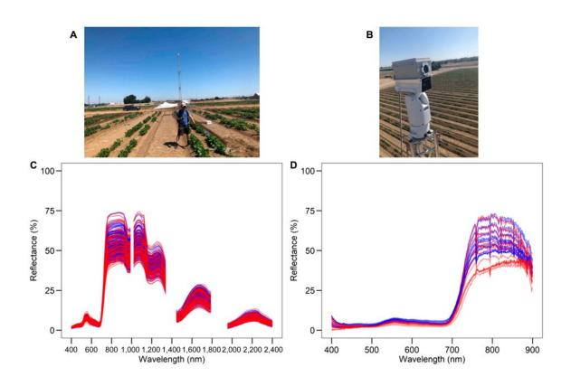
Hyperspectral reflectance of beans from ground-based (A and C) and tower-based instruments (B and D) for control (blue) and drought (red) treatments. Credit: Christopher YS Wong et al. from University of California, Davis
