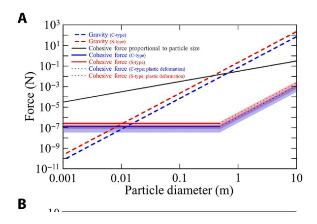
Low cohesive force and high surface mobility of asteroid particles. (A) Comparison of gravity and cohesive forces acting on particles on the surfaces of
