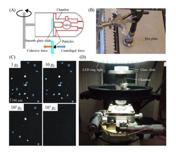
Configuration of cohesive force measurements under reduced pressure. (A) Schematic diagram of centrifugal force application under reduced pressure. The cohesive force of particles was measured under reduced pressure in a space
