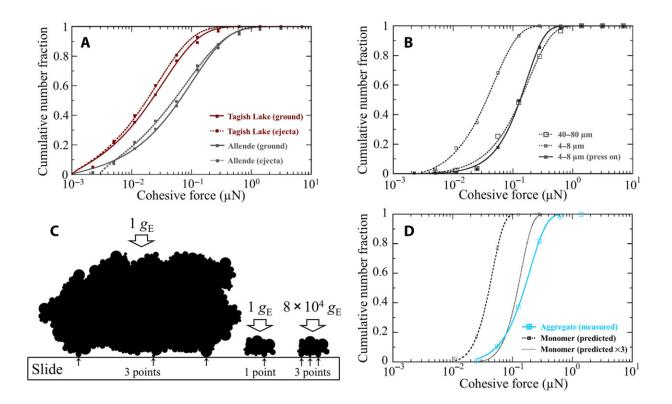
Cohesive force of particles. (A) Measured cohesive force of Allende and Tagish Lake meteorite fragments, prepared by a mortar and pestle or projectile impact, against a smooth glass slide under ambient conditions. The fitted curves were
