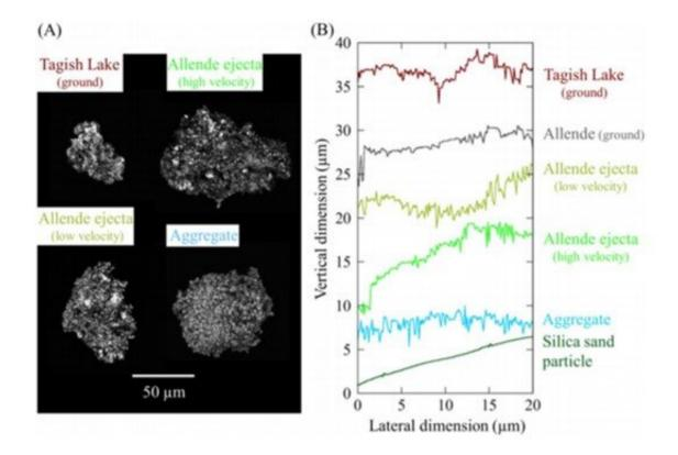
Microscopic morphology of particle. (A) Surface morphologies of each type of sample particle acquired via confocal laser scanning microscopy, and (B) onedimensional profile extracted from the data. The horizontal axis shows the location along a line perpendicular to the line of sight, and the vertical axis shows the height. Data for the Allende ground fragment and silica sand particle are from a previous study. Credit: *Science Advances* (2023). DOI: 10.1126/sciadv.add3530
