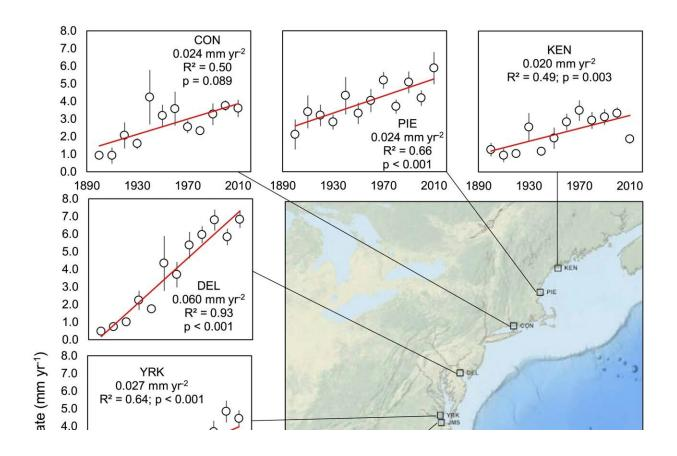
Composite (from 3 or 4 soil cores in each system) decadally averaged (±SE) rates of vertical accretion (?) from 1900s to the 2010s at nine tidal wetland sites along the U.S. East Coast with the site-average linear acceleration in accretion (; mm yr<sup>-2</sup>) denoted by the best-fit line. Credit: *Earth's Future* (2023). DOI: 10.1029/2022EF003037
