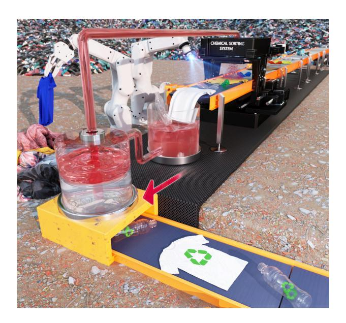
Chemical sorting can be utilized to selectively collect polyester from waste plastics and textiles. In the product stream, clean polyesters are obtained because the process eliminates colorants and most organic impurities as well. Credit:
