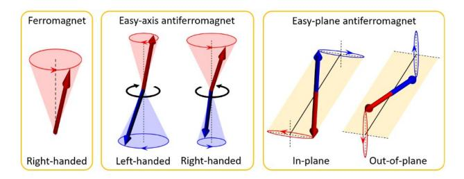
Fig. 2. Coherent spin dynamics (magnon modes) of a ferromagnet (right-handed mode), an easy-axis collinear antiferromagnet (left-handed and right-handed modes), and an easy-plane collinear antiferromagnet (in-plane and out-of-plane modes). Credit: Tohoku University
