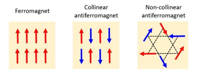
Fig. 1. Spin structures of a ferromagnet, a collinear antiferromagnet, and a noncollinear antiferromagnet. Credit: Tohoku University
