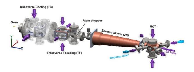
Schematic diagram of an ATTA apparatus for <sup>41</sup>Ca/Ca analysis. Credit: XIA Tongyan et al.
