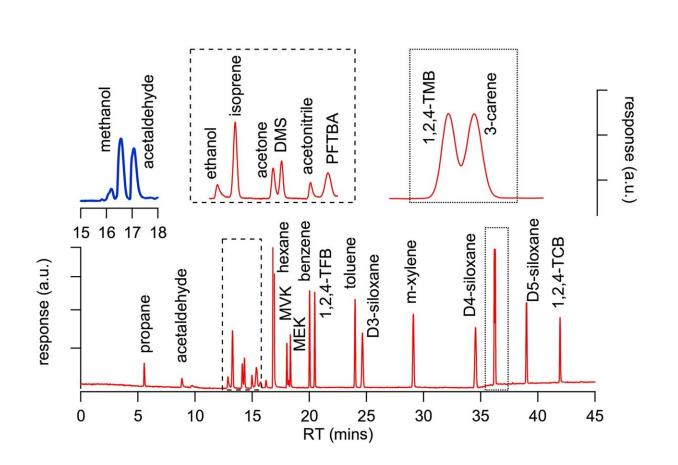
Chromatogram of PRM 0819 showing separation of compounds in the GC-FID/MS (red trace) and Cryo-GC-FID (blue trace). Credit: *Atmospheric Measurement Techniques* (2023). DOI: 10.5194/amt-16-1061-2023
