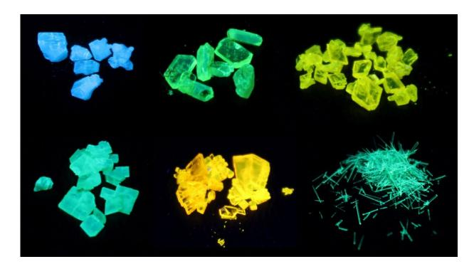
Selected crystals of phosphole-based materials under UV light (395 nm). Credit: Nils König
