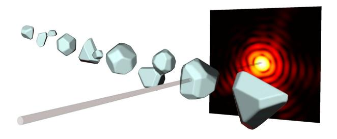
From the diffraction patterns (red) of X-ray pulses (grey), with which nanoparticles are bombarded, researchers at ETH can calculate three-dimensional images. Credit: ETH Zürich / Daniela Rupp
