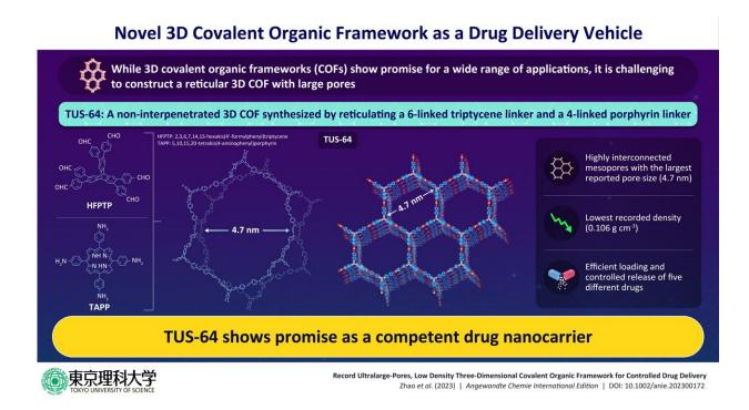
TUS scientists have synthesized a novel 3D COF, TUS-64, with the largest recorded pore size by combining a 6-linked triptycene linker and a 4-linked porphyrin linker. With a stable and highly interconnected structure, TUS-64 enables efficient drug storage and their controlled release. Credit: Yuichi Negishi from TUS, Japan
