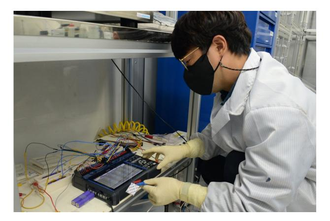
ETRI researcher is measuring the performance of a lithium-ion batteries to which fluorosulfate-based flame retardant additives are applied. Credit: Electronics and Telecommunications Research Institute(ETRI)
