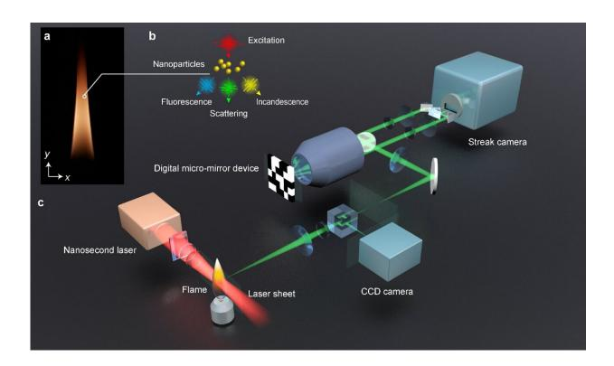
a, A photograph of the kerosene flame studied in this work. b, Illustration of three optical signals when nanoparticles (e.g. soot, PAH molecules) in the flame interact with the nanosecond laser-sheet. These signals include laser-induced fluorescence, laser-induced incandescence, and scattering. c, Schematic of the LS-CUP imaging system. Credit: Yogeshwar Nath Mishra, Peng Wang, Florian Bauer, Yide Zhang, Dag Hanstorp, Stefan Will, and Lihong V. Wang
