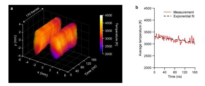
a, Spatiotemporal dynamics of flame temperature when excited by a single nanosecond light pulse. The temperature is calculated by taking laser-induced incandescence signals from two distinct color channels. b, Spatially averaged temperature evolution and its exponential fit, showing a rapid cooling after laser excitation. Credit: Yogeshwar Nath Mishra, Peng Wang, Florian Bauer, Yide Zhang, Dag Hanstorp, Stefan Will, and Lihong V. Wang
