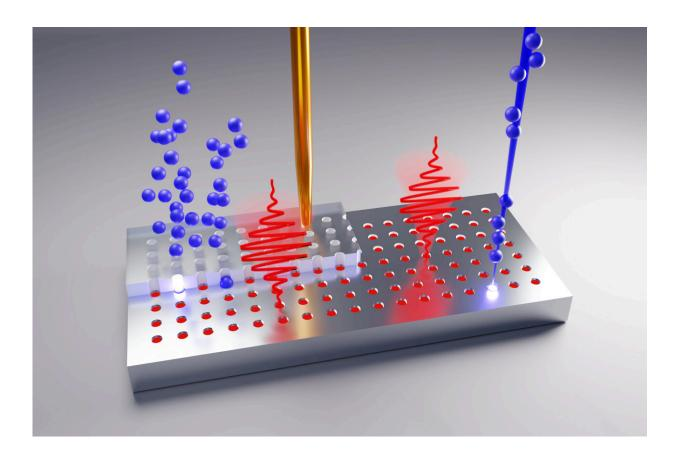
Controlled generation of single-photon emitters in silicon by broad-beam implantation of ions through a lithographic mask and by a scanned focused ion beam. Symbolically shown: the emission of two single photons. Credit: B. Schröder/HZDRM
