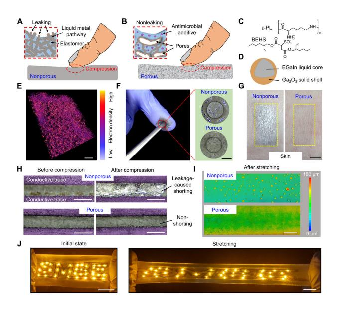
Leakage-resistant property. Conceptual illustration of conventional nonporous (A) and multifunctional porous (B) EGaIn composites upon compression. Here,
