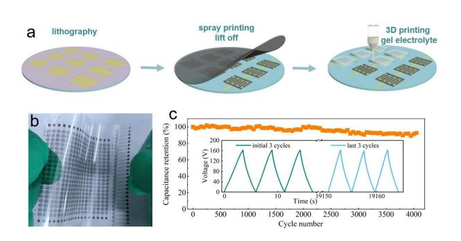
(a) Schematic of the fabrication of M-MIMSCs. (b) Flexibility of M-MIMSCs on a flexible polyethylene terephthalate substrate. (c) Cycling stability for 4000 cycles tested at 2.7  $\mu$ A of 60 cells connected in series under output voltage of 162 V in PVDF-HFP-EMIMBF4 gel electrolyte. Photo credit: Dr. Sen Wang and Dr. Linmei Li. Credit: Science China Press
