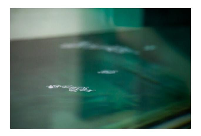
Microplastic pellets float on the surface of water in the wind wave tank at the U-M Marine Hydrodynamics Laboratory. Credit: Robert Coelius/Michigan Engineering
