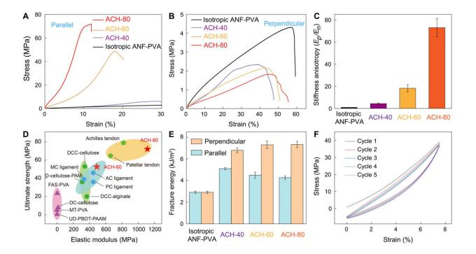
Mechanics of ACHs. (A and B) Tensile stress-strain curves of ACHs in the directions parallel (A) and perpendicular (B) to the fiber orientation, respectively, as compared with the responses of isotropic ANF-PVA hydrogels. The sample denoted as ACH-x corresponds to x% of imposed elongation during
