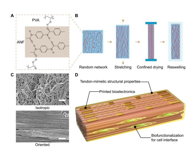
Design and processing of tendon-mimetic anisotropic composite hydrogels (ACHs). (A) Chemical structures of ANF and PVA and their intermolecular hydrogen bonding. (B) Schematics of the processing steps for ACH involving stretching and confined drying for the orientation of nanofiber assembly. (C) SEM images of isotropic ANF-PVA hydrogel (top) and ACH-80 (bottom). Scale bars, 1 µm. (D) Schematics of the multifunctional tendon-mimetic ACHs.
