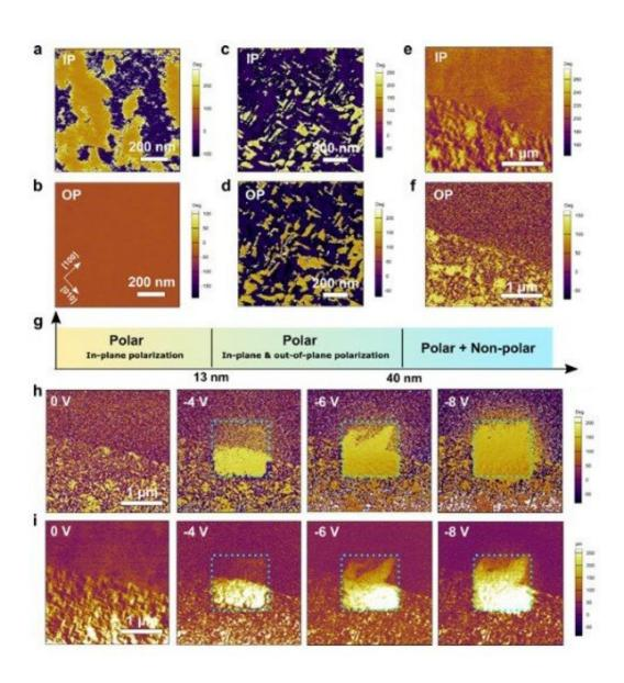
Piezoresponse force microscopy (PFM) of emergent ferroelectricity and phase coexistence in NaNbO<sub>3</sub> membranes. Lateral and vertical PFM phase images obtained for a) and b) 13 nm, c) and d) 40 nm, and e) and f) 100 nm thick
