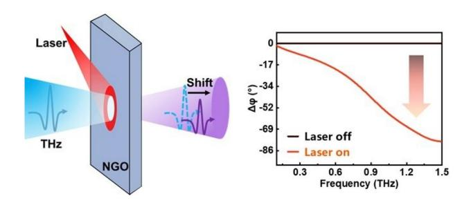
Schematic diagram of terahertz modulation experiment and phase shift as a function of terahertz frequency and light switch. Credit: Xu Jinyi
