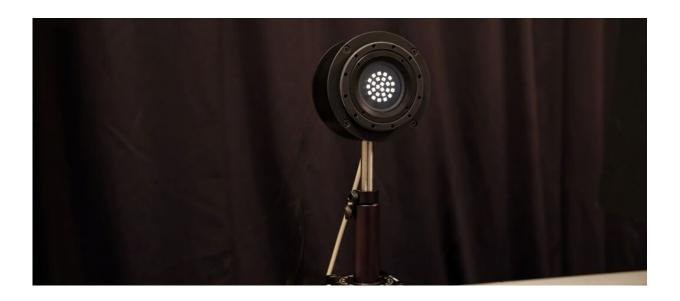
LED-based light source developed in PhotoLED project. The LED chips have been selected to produce a spectrum of light resembling the new reference spectrum CIE L41. Credit: Tuomas Poikonen / VTT
