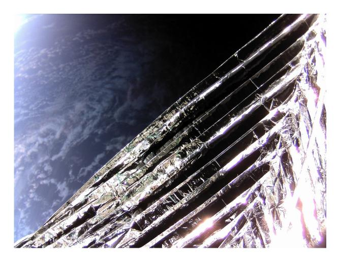
The deployment of the Drag Augmentation Deorbiting System (ADEO) was captured in front of the 'eyes' of the integrated camera onboard the ION satellite carrier, as ADEO unfurled showing its 'wings', and immediately initiated the satellite's descent. The image shows one edge of the sail—a large aluminumcoated polyamide membrane attached to four carbon-fiber reinforced booms, following its jack-in-a-box deployment. Credit: ESA
