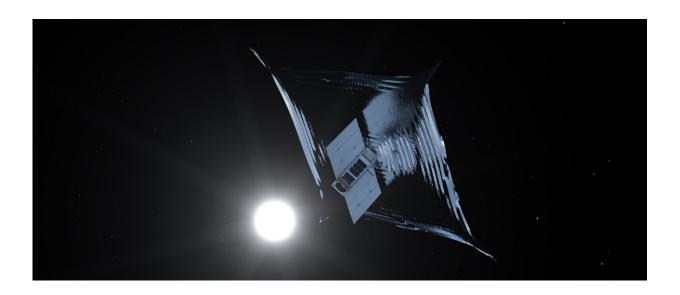
Artist impression of the Drag Augmentation Deorbiting System (ADEO) breaking sail. A drag breaking sail can provide a passive method of deorbiting by increasing the atmospheric surface drag effect and causing an accelerated decay in the satellite's orbital altitude. The satellite will eventually burn up in the atmosphere, providing a quicker residue-free method of disposal. Credit: ESA
