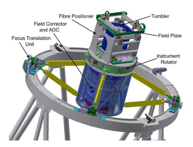
A computer-aided diagram (CAD) representation of the WEAVE top-end assembly, incorporating the prime-focus (field) corrector system, instrument rotator and fiber positioner. The four mounting units on the outer ring of the telescope structure provide for focus and tilt correction of the whole system. Credit: arXiv (2022). DOI: 10.48550/arxiv.2212.03981
