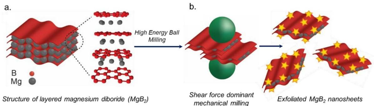
Synthesis scheme: (a) structure of bulk  $MgB_2$ ; (b) the exfoliation of  $MgB_2$  using a high-energy ball mill to obtain exfoliated  $MgB_2$  nanosheets with active sites (gold stars). Credit: *Small* (2022). DOI: 10.1002/sml.202205487
