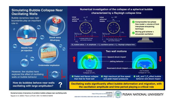
Researchers from Korea and Vietnam simulate the dynamics of bubble collapse near oscillating walls in a new study, showing that the bubble collapse in such a case has high maximum flow speed and peak impact pressures. Their findings could help resolve microjet direction and cavitation erosion control problems. Credit: Prof. Warn-Gyu Park from PNU, Korea.
