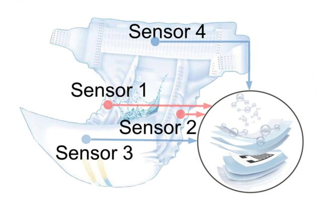
A Penn State-led research team integrated four humidity sensors between the absorbent layers of a diaper to create a "smart diaper," capable of detecting wetness and alerting for a change. Credit: Huanyu "Larry" Cheng/Penn State
