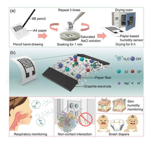
Illustration showing fabrication and application of the pencil-on-paper hydration sensor. Schematics showing the (a) fabrication processes and (b) the response mechanism of the flexible pencil-on-paper hydration sensor with (c) applications in health monitoring, noncontact switching, and skin characterizations. Credit: Huanyu "Larry" Cheng / Penn State
