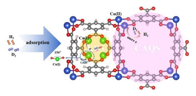
The separation mechanism of  $D_2/H_2$  mixture in Cu(I)Cu(II)-BTC. Credit: by Hu Xiaoyu
