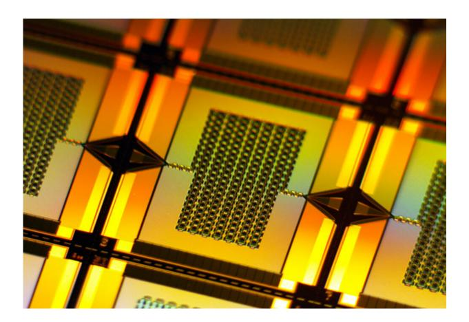
This superconducting parametric amplifier can achieve quantum squeezing over much broader bandwidths than other designs, which could lead to faster and more accurate quantum measurements. Credit: Jack Qiu, William D. Oliver, and Kevin P. O'Brien
