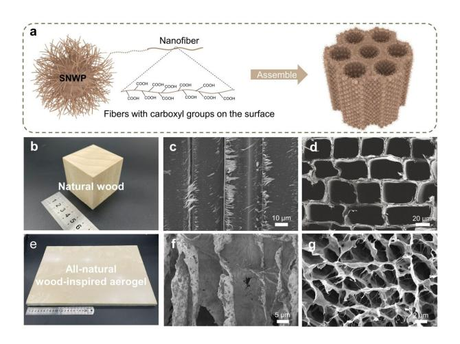
A schematic diagram shows the structure of the all-natural wood-inspired aerogel. Credit: University of Science and Technology of China
