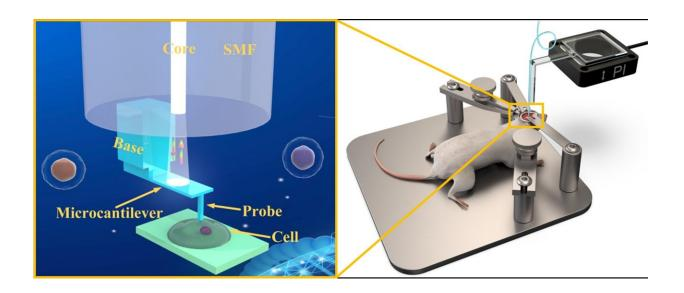
Fiber optical nanomechanical probe (FONP) fabricated by femtosecond laser two-photon polymerization technology can realize the biomechanical measurement down to 2.1 nanonewton. Such high precision enables the measurement of in vivo biomechanical properties of tissue, single cell, and other soft biomaterials. Credit: *International Journal of Extreme Manufacturing* (2023). DOI: 10.1088/2631-7990/acb741
