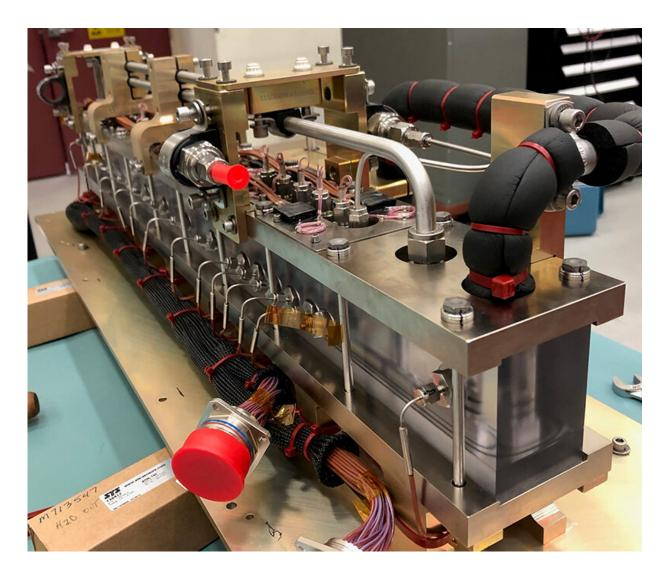
Purdue University engineers conducted the first phase of the Flow Boiling and Condensation Experiment using the Flow Boiling Module, which gathered data on how boiling happens in reduced gravity. Pictured here is this module prior to being launched for installation on the International Space Station. Credit: NASA Glenn Research Center
