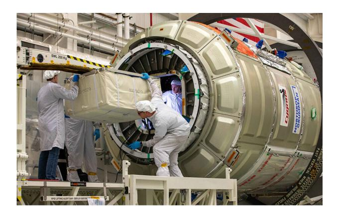
An experiment designed by Purdue University researchers to study the effects of reduced gravity on boiling is loaded onto a Cygnus spacecraft in preparation for launch onboard an Antares rocket to the International Space Station. Credit: Northrop Grumman/NASA
