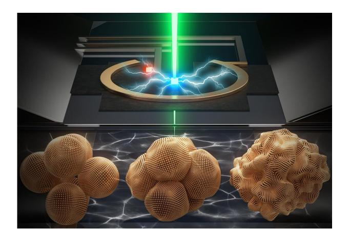
Artist's rendering of a copper nanoparticle as it evolves during CO2 electrolysis: Copper nanoparticles (left) combine into larger metallic copper "nanograins" (right) within seconds of the electrochemical reaction, reducing CO2 into new multicarbon products. Credit: Yao Yang/Berkeley Lab
